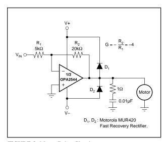
FIGURE 3. Motor Drive Circuit.
