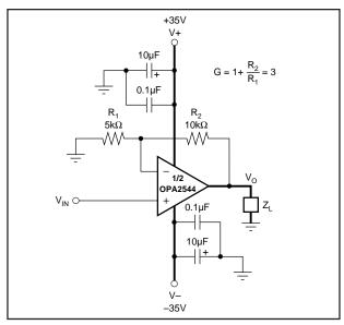
FIGURE 1. Basic Circuit Connections.
