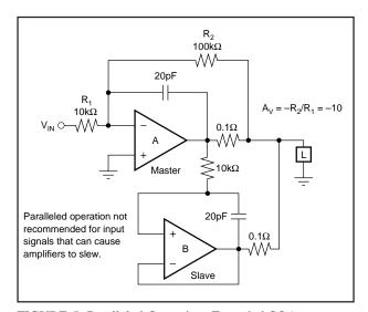
FIGURE 5. Paralleled Operation, Extended SOA.
