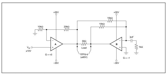
FIGURE 4. Bridge Drive Circuit.
