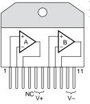
Case connected to V– Supply.
